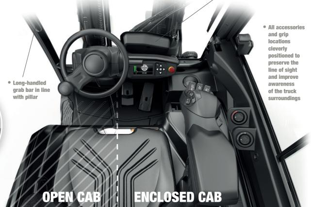
• Seat, steering wheel and dashboard positions optimised for front visibility
